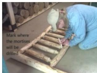
**TIP** After your tenons are cut, lay all parts out to mark where to drill your tenons. In addition to marking where the mortise is to be drilled, You might also want to make pencil marks on the side to indicate the drill angle to refer to when drilling the mortise.
