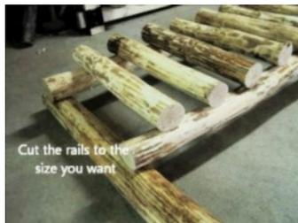
**TIP** After you have cut the tenons, mark the rails where you will be drilling the mortises. At this point also pay attention to the lengths of the rails, as some may need to be trimmed. If your rail is curved, you might also want to pencil an angle line to remember what angle the mortise is to be drilled.
