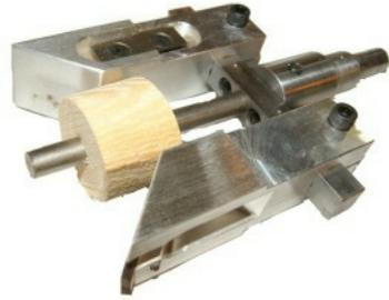
**TIP** To make set-up blocks to quickly set up tenon diameter, just make one extra long tenon and cut a little chunk off the end. Mark what size it is and put it in a safe place where it won't get thrown away by mistake. When you need to set your cutter up for that specific sized tenon again, simply slide that piece of tenon onto the guide bar of the cutter and slide the cutter arms in until the blades touch the block and tighten the arms.
