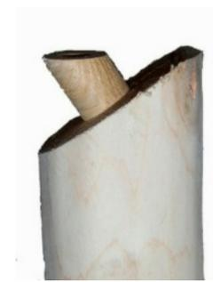
After you have drilled the pilot hole, put the E-Z Tenon Cutter into your drill, secure, and insert the guide bar into the pilot hole. Start drilling slowly until the edges of the log are cut. Gradually add more pressure to finish cutting the tenon
