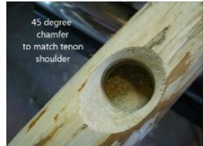
The E-Z Sink is NOT a drill bit. It is a countersink bit. You must first drill the mortise using either a 1.5" or 2" flat spade drill bit, or a forstner bit. The E-Z Sink is then inserted into the mortise. Slowly start your drill so that the blades start shaving off the edges of the mortise. The depth of the countersink will be determined by how deep you drilled your mortise.
