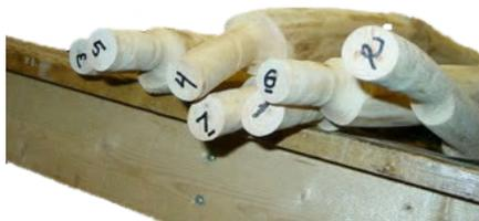
**TIP** It is best to work with dry wood. If you must work with green wood, be aware that the tenons may shrink or crack when they dry, which may eventually cause the joint to loosen. For small diameter tenons, it is a good idea to glue in a piece of 3/8" wood dowel into the pilot hole for added strength.
